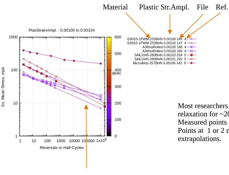
Most researchers only measured relaxation for ~200 or 1000 cycles. Measured points are shown. Points at 1 or 2 million are from extrapolations.
