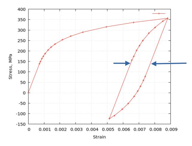
Measure the width of the loop. This is the Plastic Strain **Range**.
