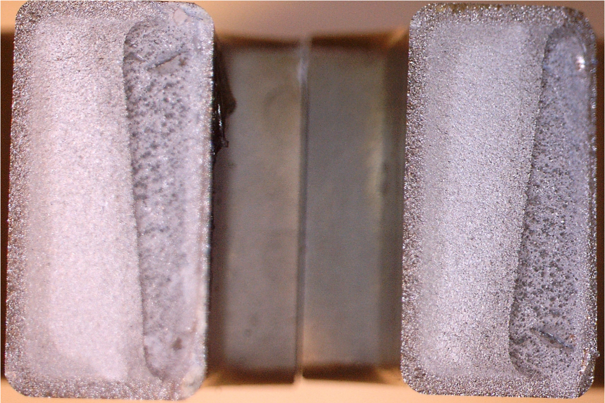
Figure 5: Fracture surface of specimen IT201-2, 2N_f=376,820
