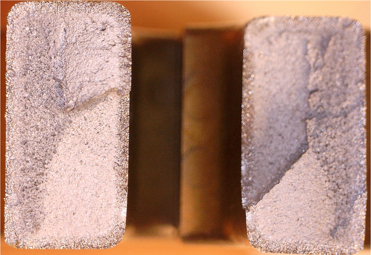
Figure 5: Fracture surface of specimen IT201A-3, 2Nf=848
