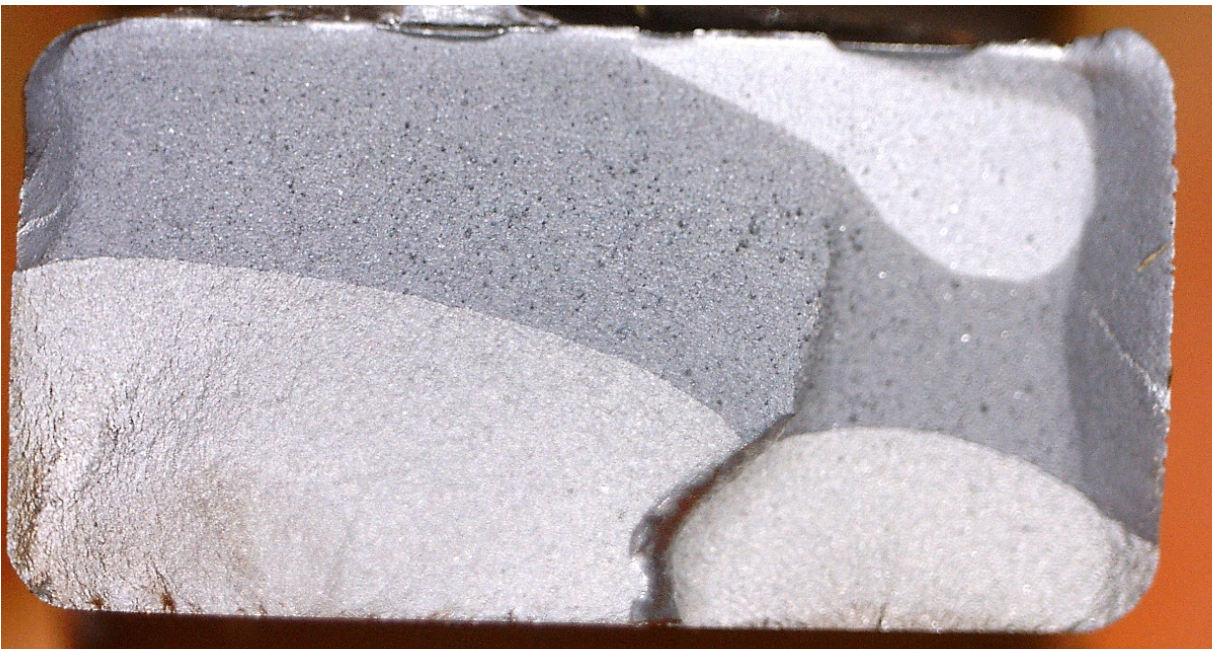
Figure 6: Fracture surface of specimen IT199-4, 2N_f=77,700
