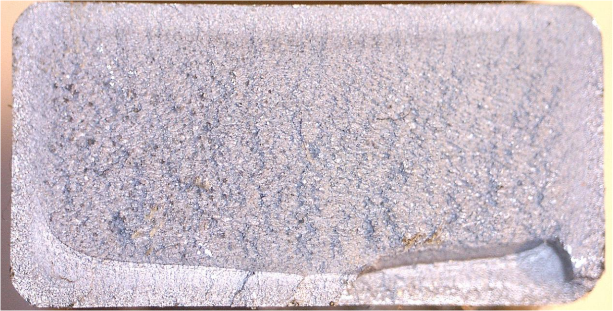
Figure 9: Fracture surface of specimen IT184-Calibration1
