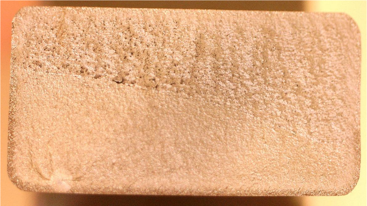
Figure 9: Fracture surface of specimen IT180-7
