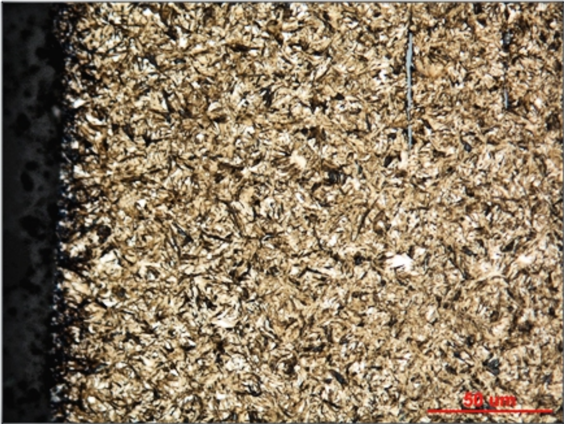
Figure 5: Microstructure of Iteration 163 & 164, case high magnification
