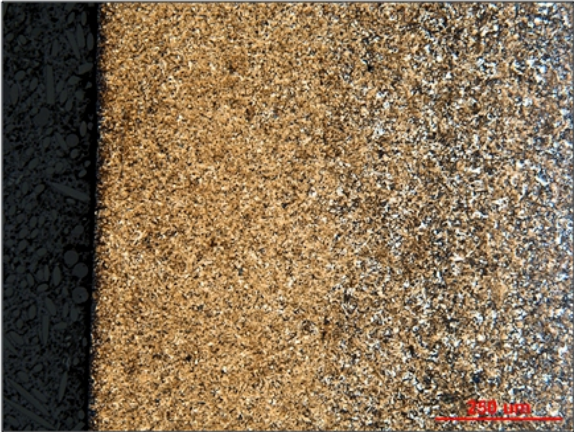
Figure 6: Microstructure of Iteration 163 & 164, case low magnification
