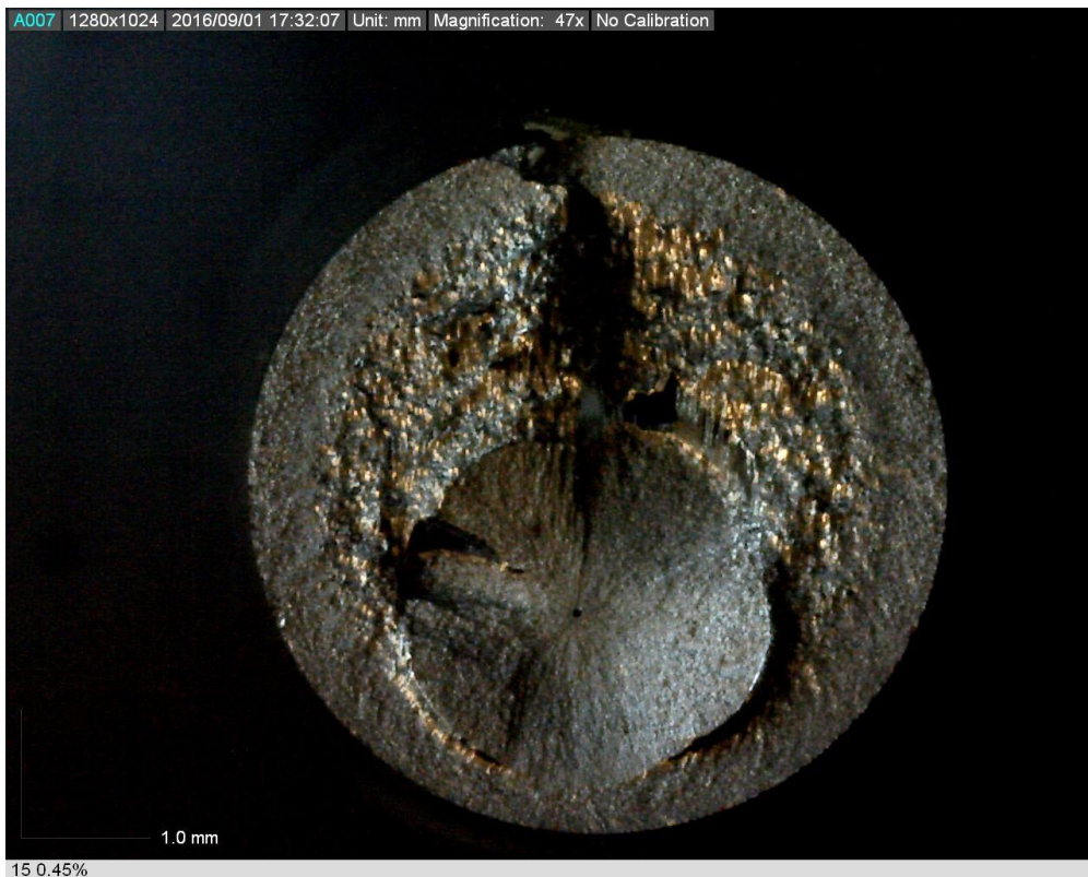
Figure C.3: Fracture surface of specimen #15 under 0.45% strain amplitude (fails with 132728 reversals )
