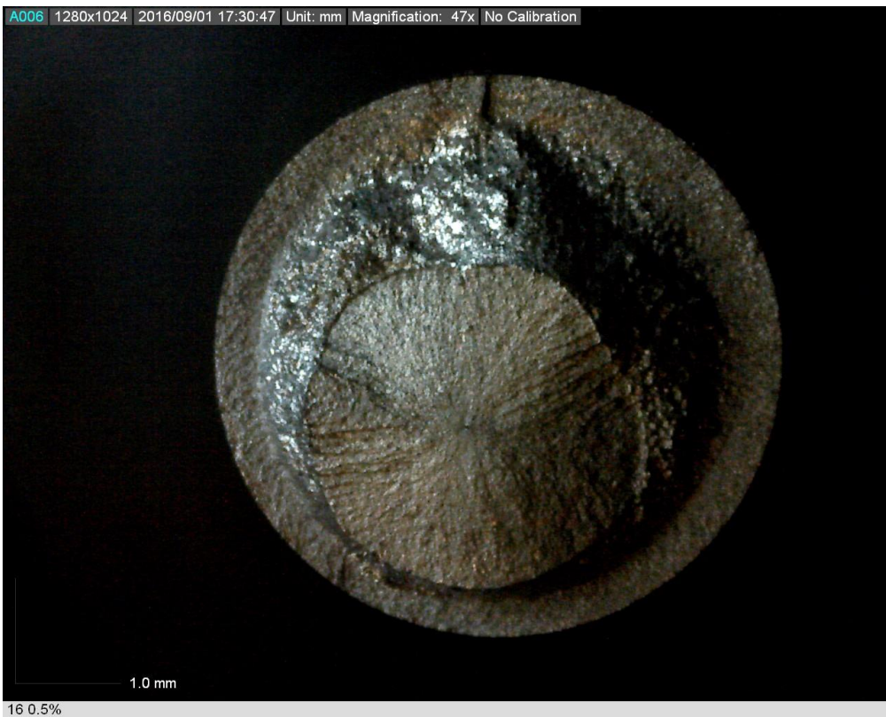
Figure C.2: Fracture surface of specimen #16 under 0.5% strain amplitude (fails with 58710 reversals )
