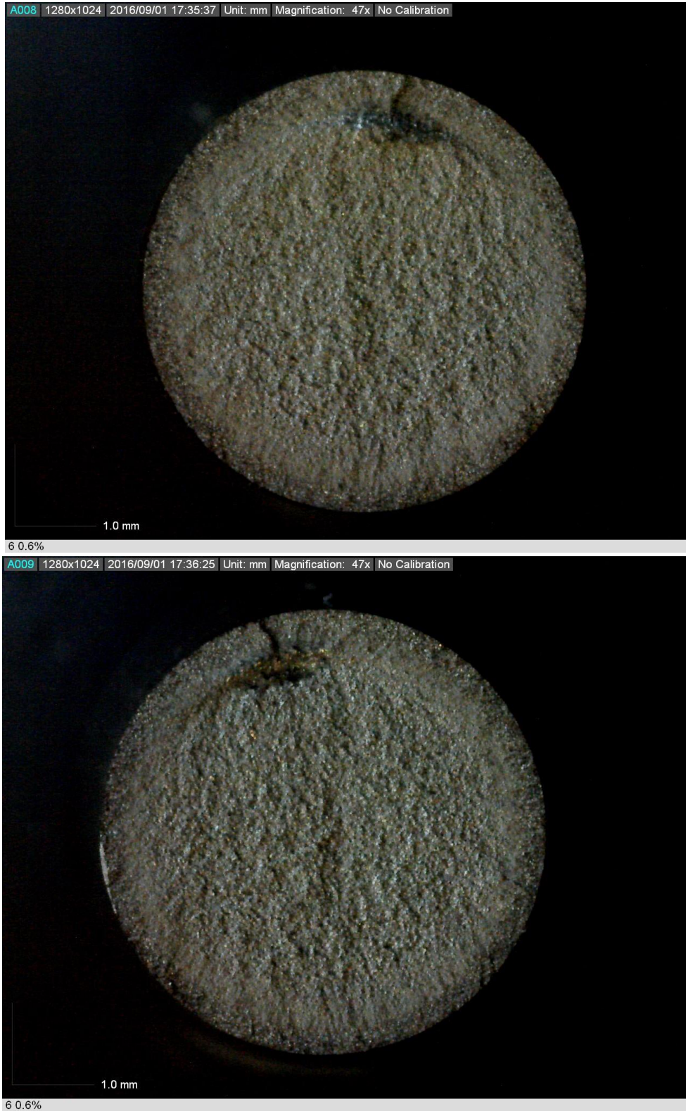
Figure C.1: Fracture surface of specimen #6 under 0.6% strain amplitude (fails with 9760 reversals )
