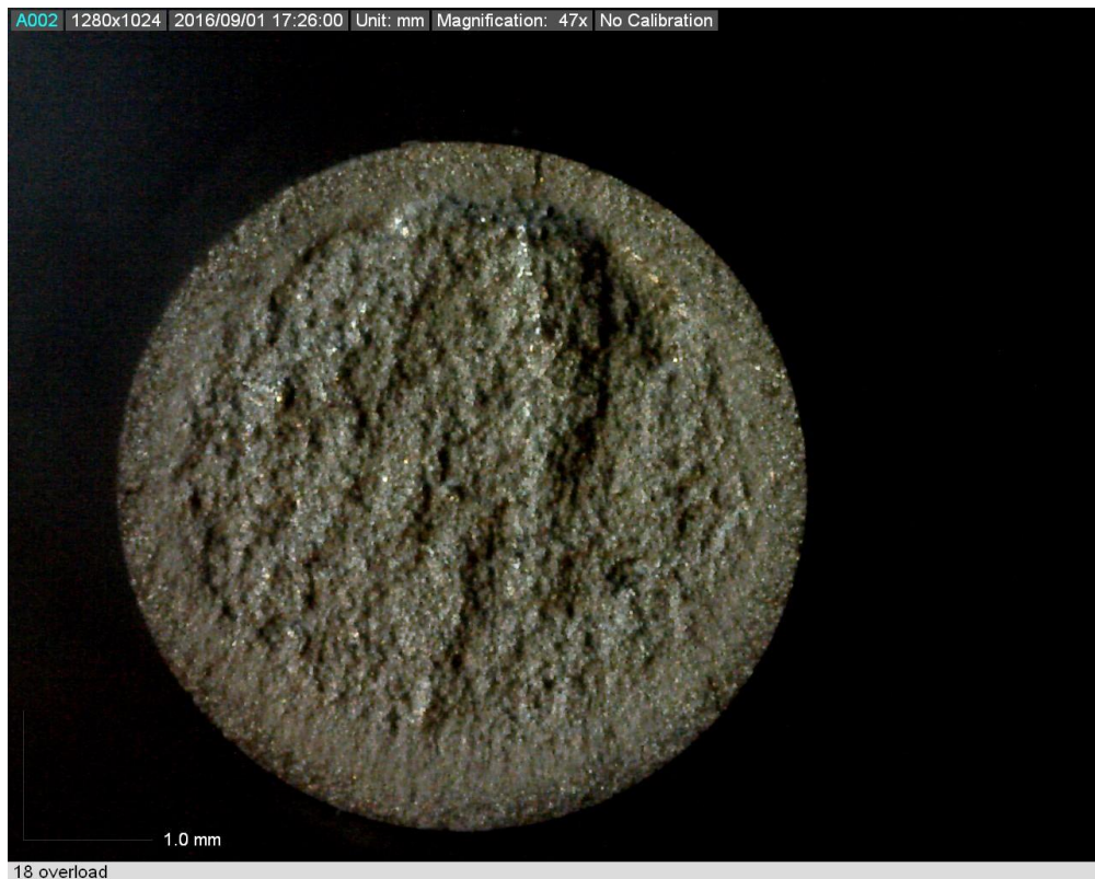
Figure C.4: Fracture surface of specimen #18 under overload
