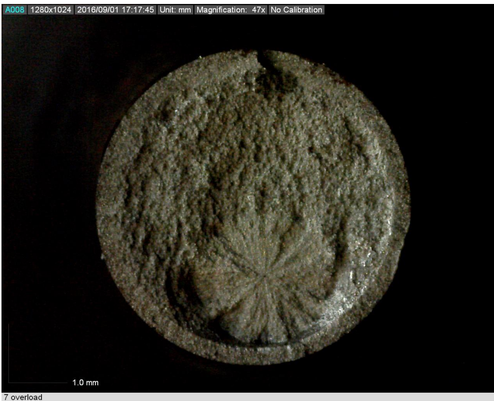
Figure C.4: Fracture surface of specimen #7 under overload
