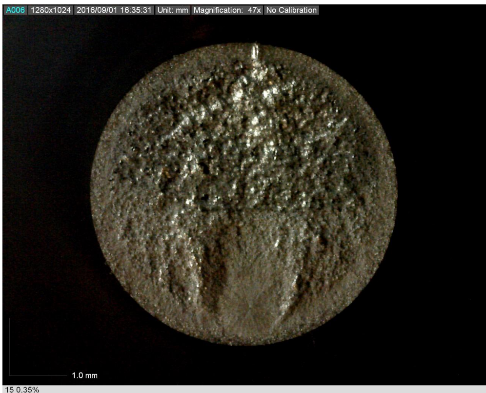
Figure C.3: Fracture surface of specimen #15 under 0.35% strain amplitude (fails with 1364932 reversals )
