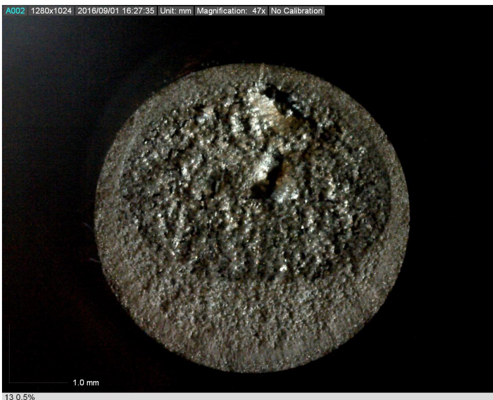
Figure C.2: Fracture surface of specimen #13 under 0.5% strain amplitude (fails with 15400 reversals )
