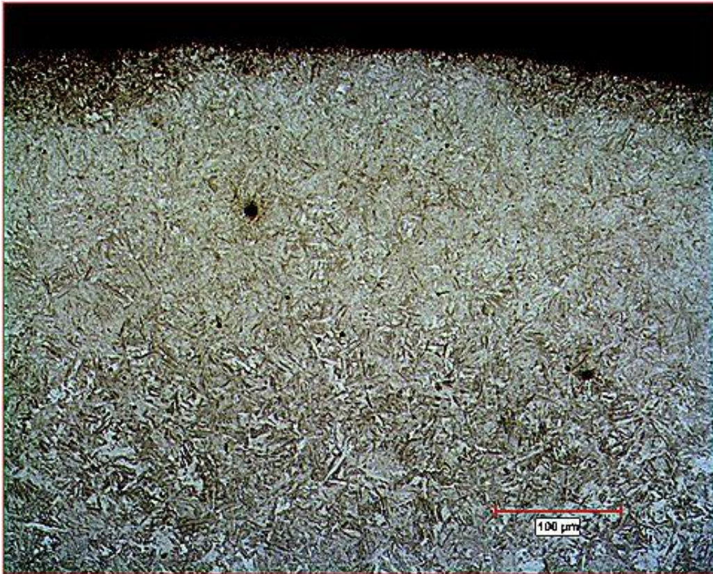
Figure 1: Low magnification photograph of the inclusion distribution in the case area (Courtesy of Chrysler)
