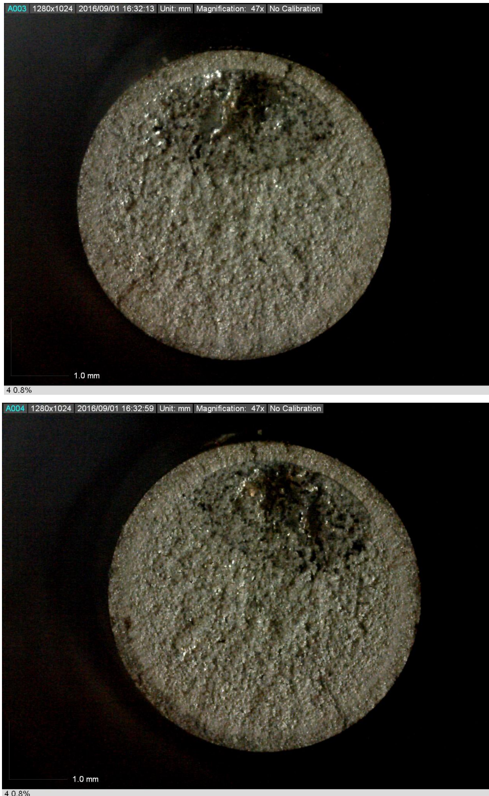
Figure C.1: Fracture surface of specimen #4 under 0.8% strain amplitude (fails with 328 reversals )
