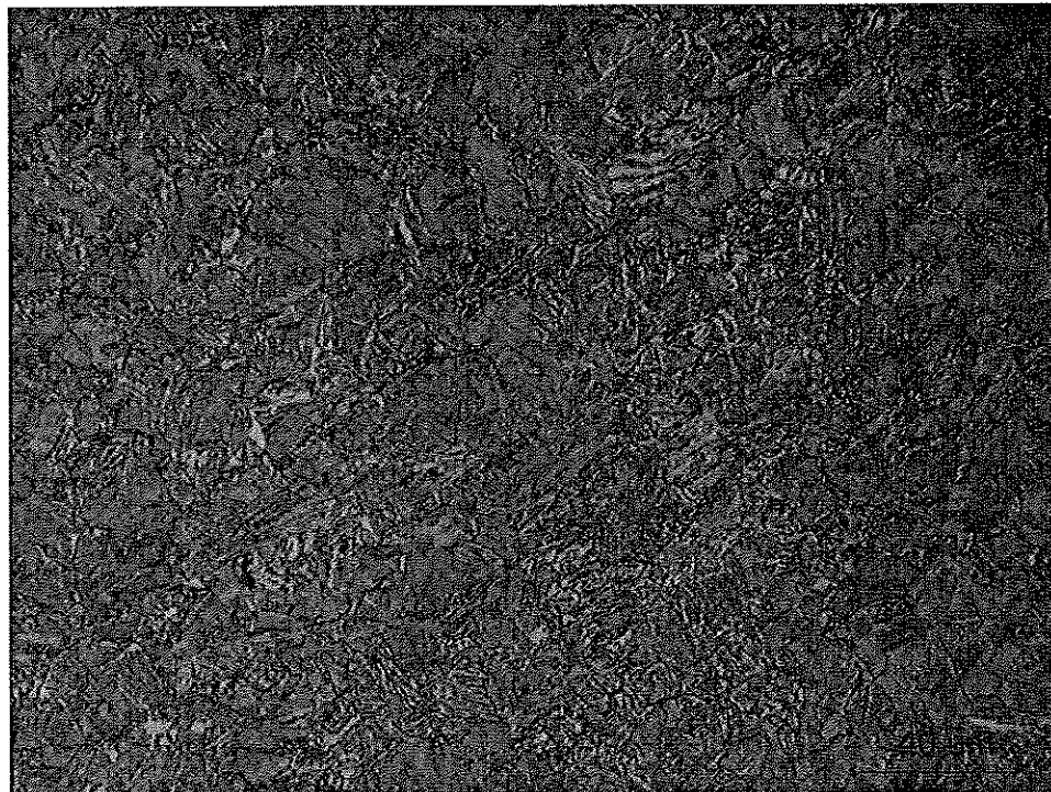
Figure 2: Micrograph at 500X magnification showing the microstructure of a longitudinal section from the grip area of a tensile specimen. (Courtesy of Chrysler)
