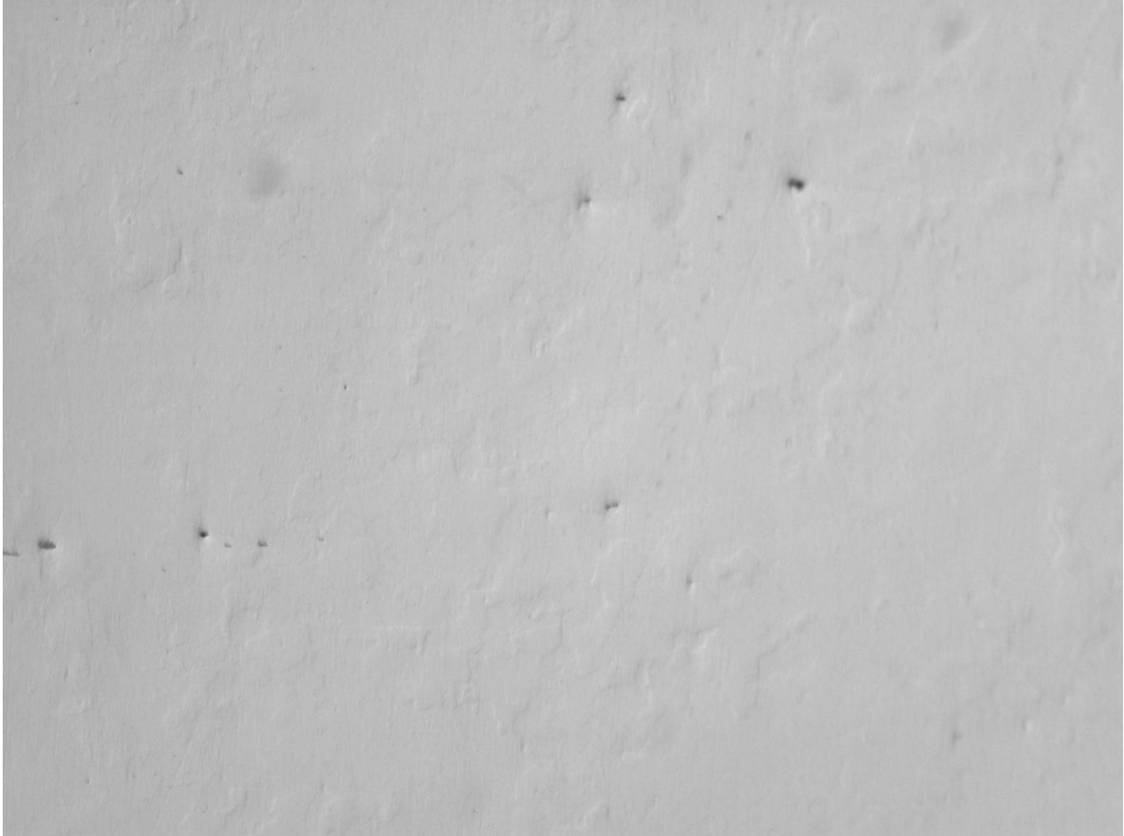
Figure 3 Inclusions 4140 induction through hardened steel (X50)
