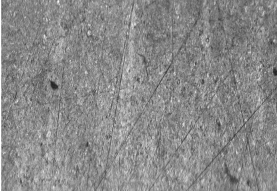
Figure 2 Photomicrographs of 5160H quenched and tempered steel (X20)
