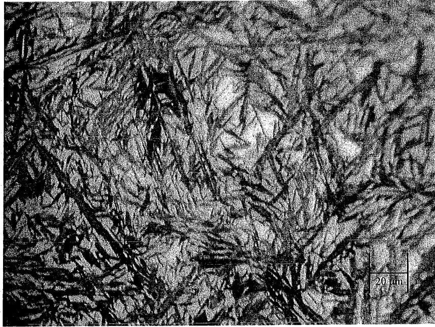
Figure 2a: Photomicrograph in the transverse direction (T-T') at 500X for SAE 86B20 Carburized Case (Vac 1700 F) steel (rolling direction is perpendicular to the page).
