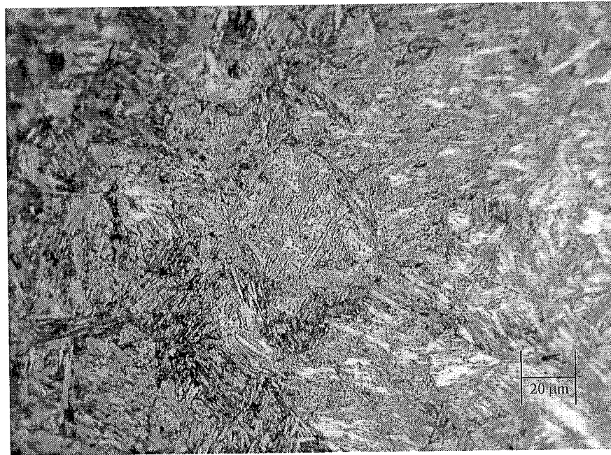
Figure 2a: Photomicrograph in the transverse direction (T-T') at 500X for SAE 41B17M (PS 19) carburized case (Vac 1800 F) steel (rolling direction is perpendicular to the page).
