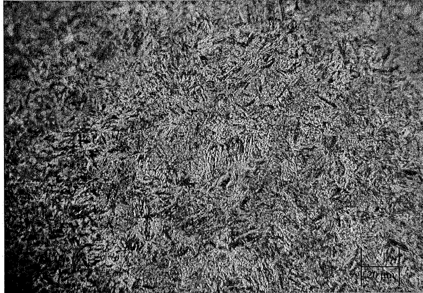
Figure 2: Photomicrograph in the transverse direction (T-T' as shown in Fig. 1c) at 500X for SAE 4140 High S (0.077% max.) steel.
