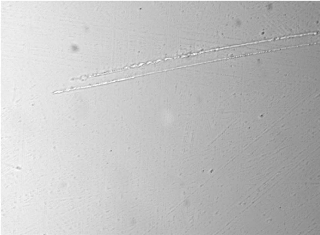
Figure 3 Inclusions photomicrograph of 4140 Quenched and Tempered steel (X100)
