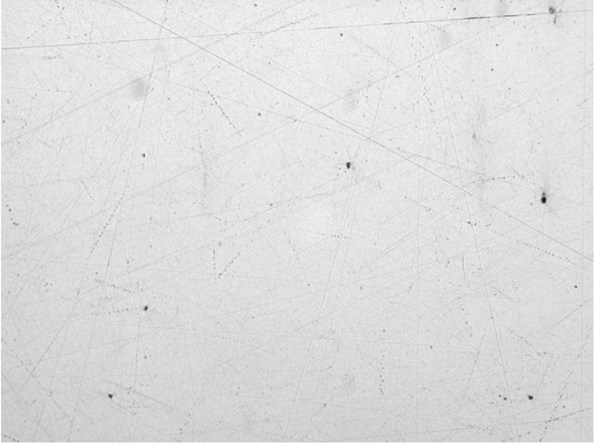
Figure 3 Inclusions photomicrograph of 9310 Quenched Core steel (X100)
