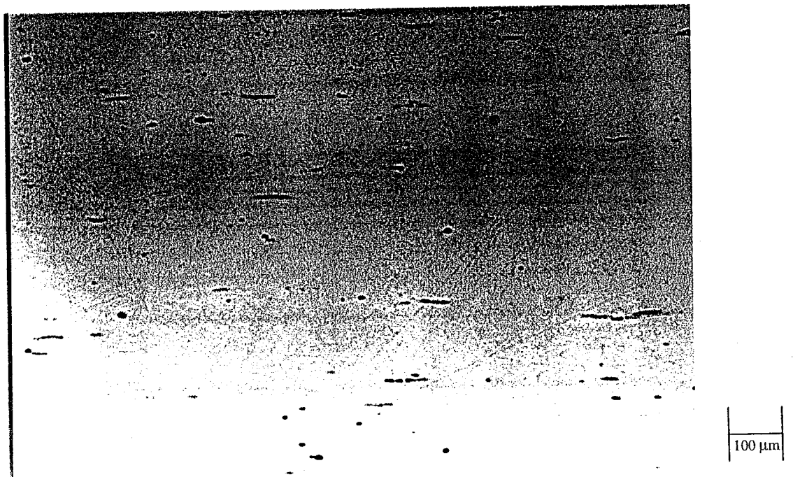
Figure 3b: Examples of inclusions in the second longitudinal direction (L-T) at 100X for SAE 10V45 deformed/FAC steel (rolling direction is horizontal)
