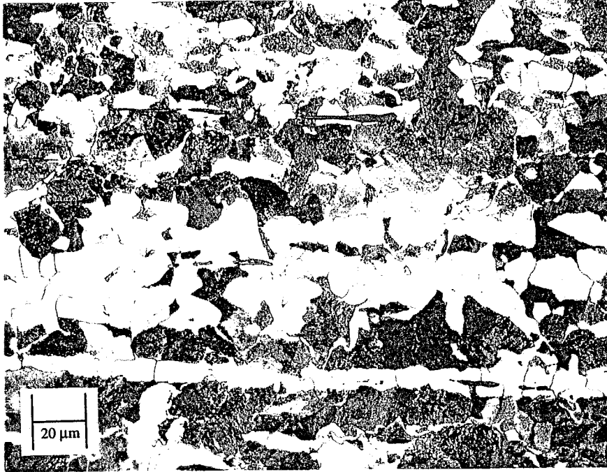
Figure 2: Photomicrograph in the longitudinal direction (L-T) at 500X for SAE 1141 (NbFG) normalized steel (rolling direction is horizontal)
