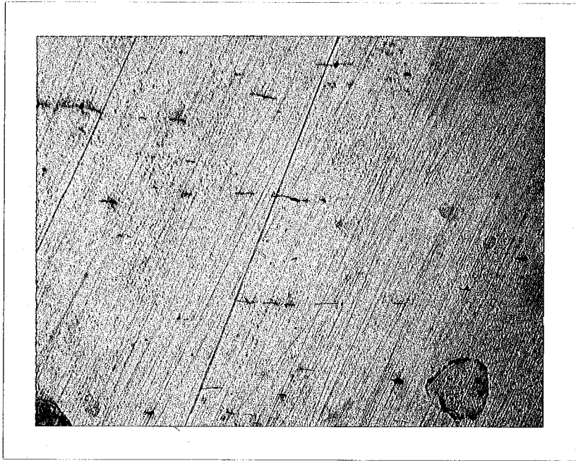
Fig. 3 Inclusions photomicrograph of AISI 1050M Induction Surface Hardened steel (X200)
