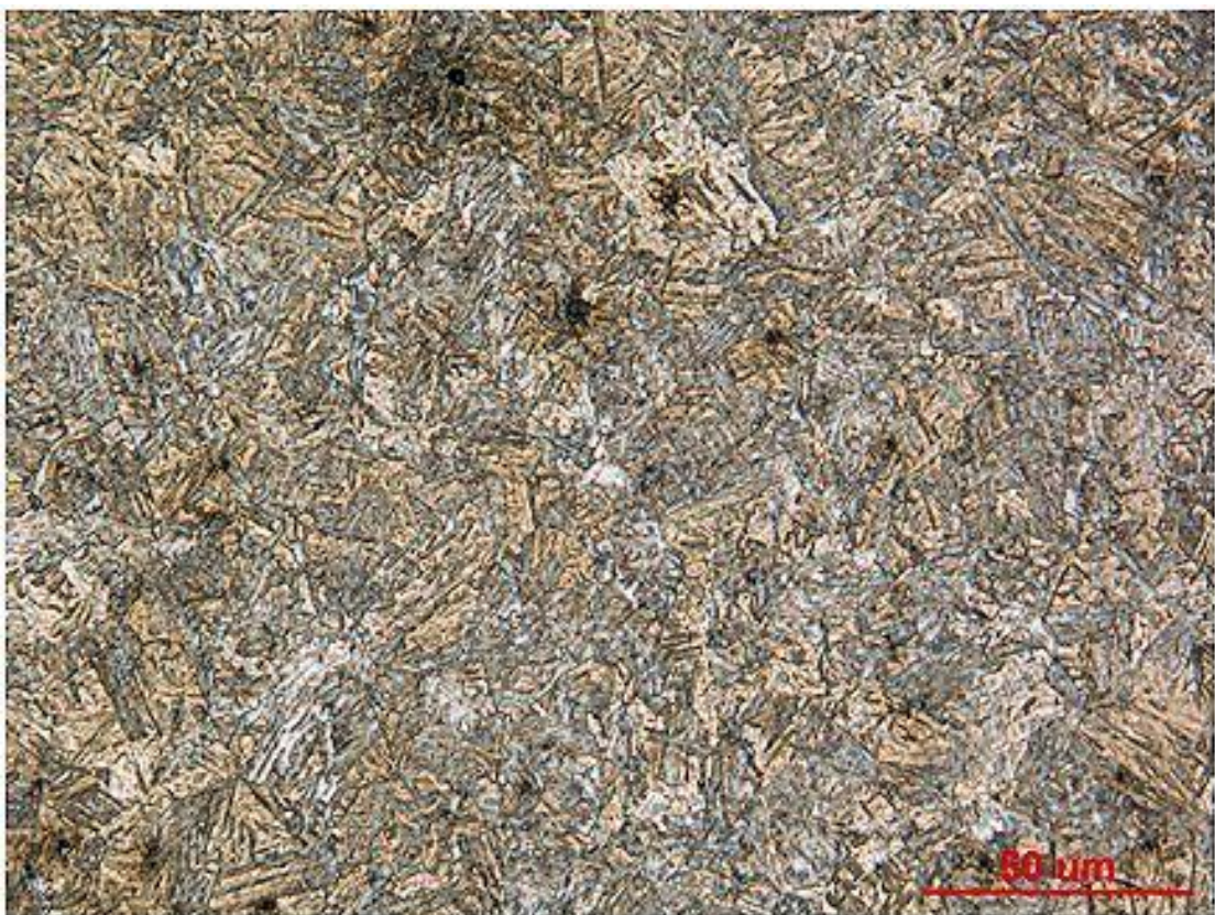
Figure 2: High magnification photo showing the microstructure of the transverse section from the gage area (Courtesy of Chrysler)
