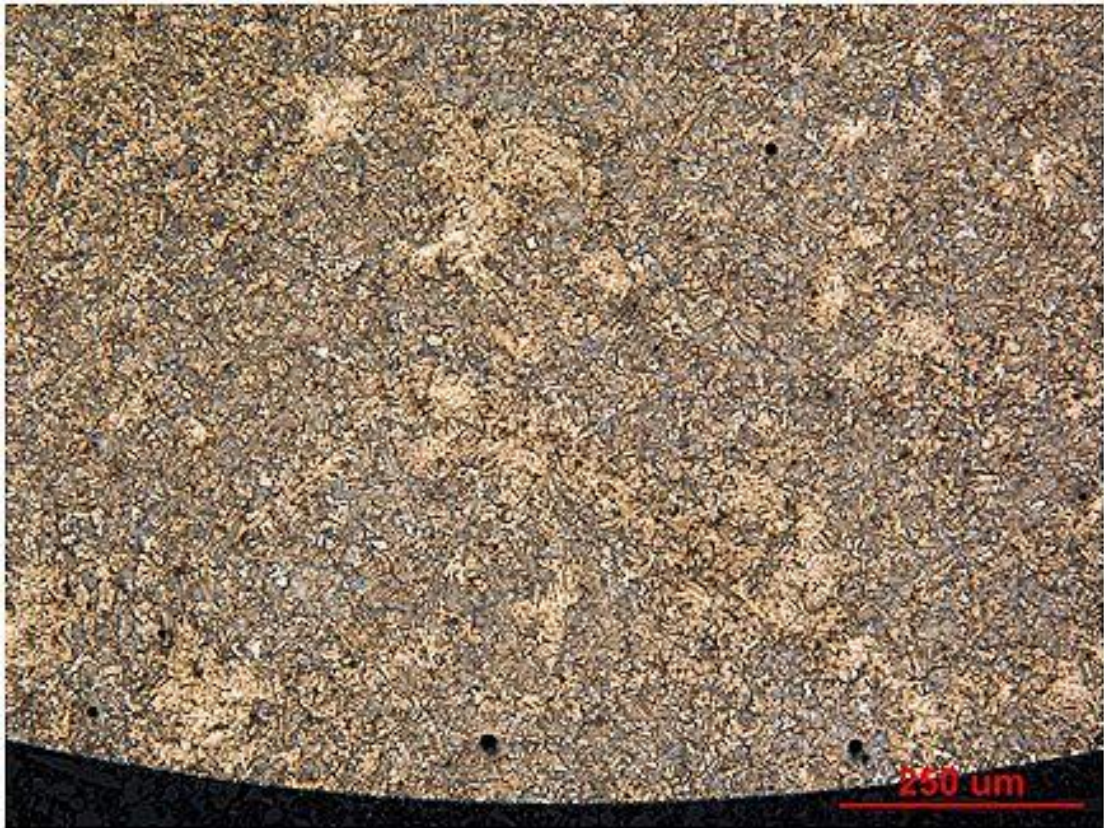
Figure 1: Low magnification photograph of the inclusion distribution in the steel (Courtesy of Chrysler)
