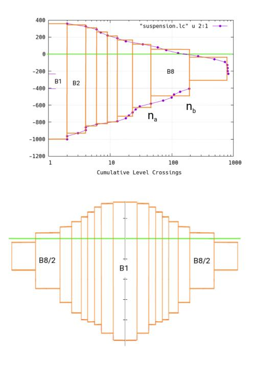
When we are given a Level count data set or plot, we can re-constitute the cycles that created it by sectioning or "blocking" the counts: Block B8 for example would have  $(n_b - n_a)$  cycles
