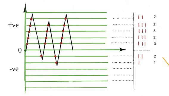
The original circuits sent a pulse to electro-mechanical counters as a signal crossed each positive voltage level.
