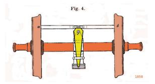
Since the zinc scratch plate was not indexed with time or mileage, the measured result would have been an observation of the max and the min loads (when calibrated) on the axle during the service test.
