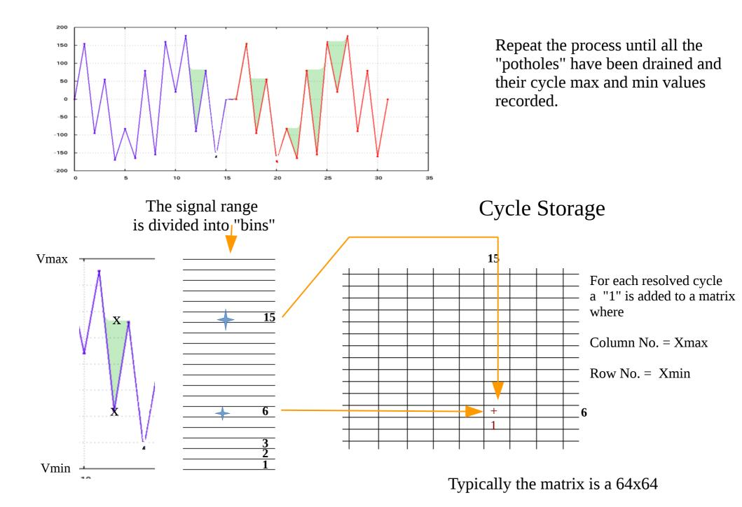
After the history has been processed the contents of the matrix are scaled back to signal value and printed to a text file with format such as: #Data column code shown below:
