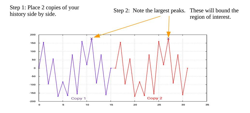
Step 3: Assume that this is the cross-section of a water reservoir. "Fill" the region between the two peaks with water.
