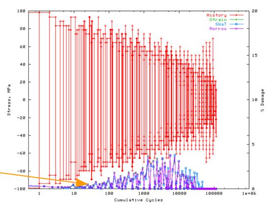
Although better than Level Crossing Counting, Rainflow Counting also has some problems that under special history conditions could lead to significant damage evaluation errors. If one imposes the strain history shown below on an axial sample the stress-strain response will show one large loop and two small ones:
