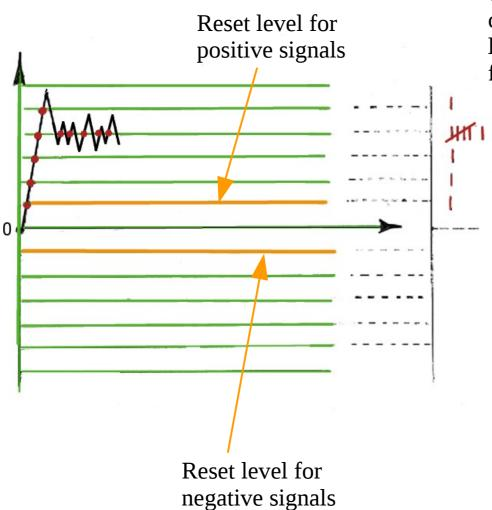
The problem of signal noise causing unexpected counts was somewhat mitigated by setting a reset level to which the signal had to return to before any further counts were allowed.
