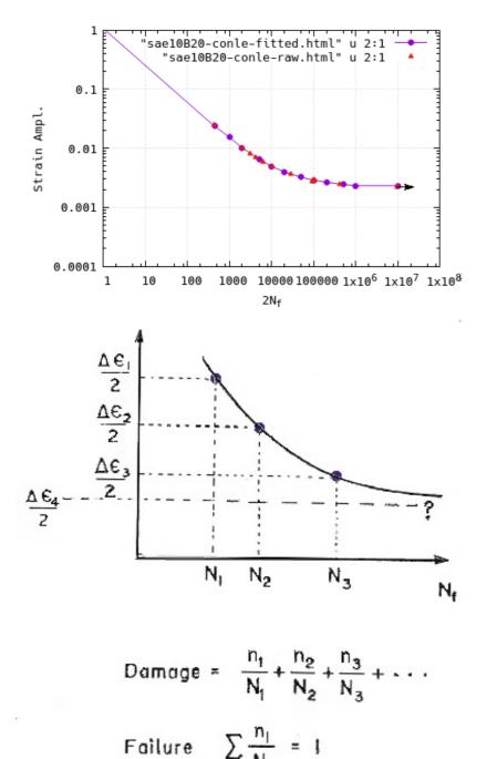
During constant amplitude (CA) testing, one generally starts with the short life specimens first and then tests the rest with the lower strains and longer lives.
