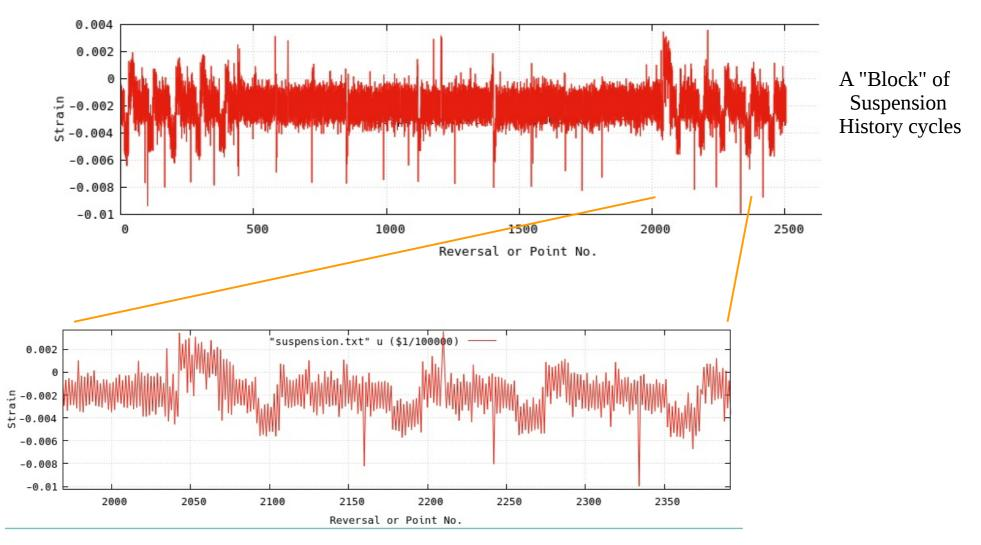
The history shown here was applied in a number of scaled down versions onto unnotched axial test samples
