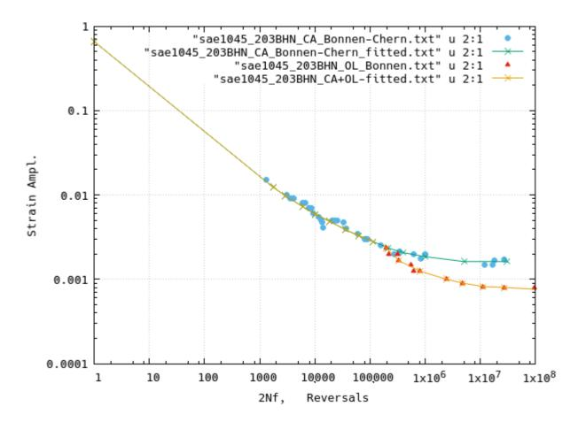
The constant amplitude and overload raw and fitted points are shown in this plot.
