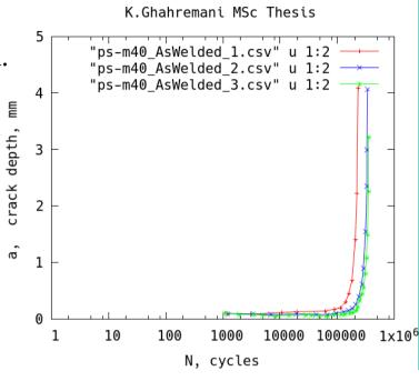
In general, as shown by Dowling\*, in long life tests crack initiation dominates, while in short life fatigue crack propagation dominates. These proportions also depend on material hardness. A very hard steel will have a very short crack propagation life.
