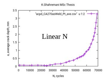
These two plots show the crack size, a vs. cycles for the same constant amplitude test.
