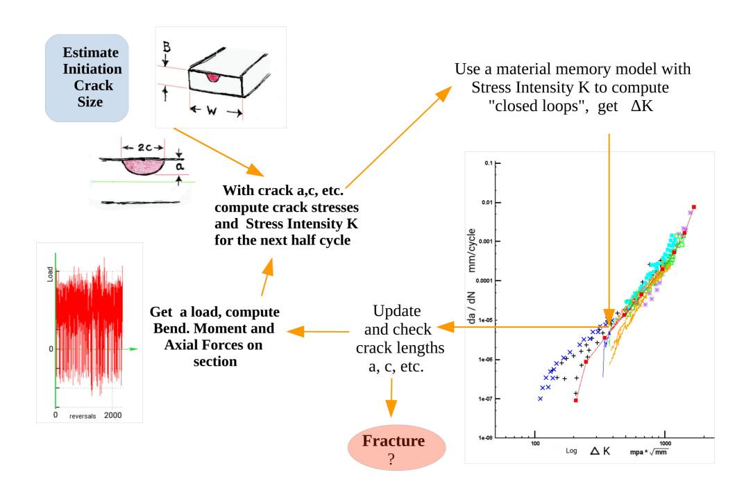
In an infinite sheet or plate with a crack the gross stress Sg applied to the sheet will cause a "Stress Intensity" K where:
