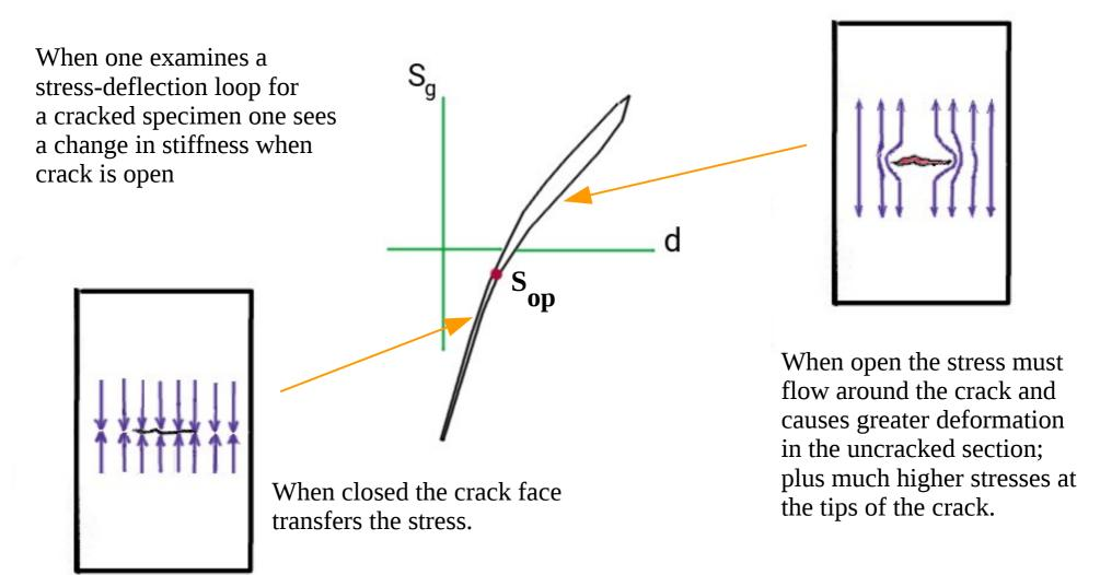
Thus an effective stress intensity, **Keff** = **Kmax** - **Kop** can be computed and used to account for the effects of mean stress cycles Plotting **da/dN** vs  $\Delta$ **Keff** helps to explain the effects of means stress (or R ratio) in crack propagation fatigue analysis, but observing the opening point in a test requires substantial experimental efforts.
