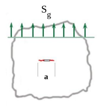
Constant amplitude specimen testing to create the basic material da/dN curves use a wide variety of geometries, but generally translate the test data into a  $\Delta K = K \max$  - Kmin.
