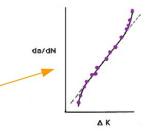
As the crack gets large the load in tension may cause the specimen to fracture. The stress intensity for this critical value is denoted as  $\mathbf{K}_{IC}$
