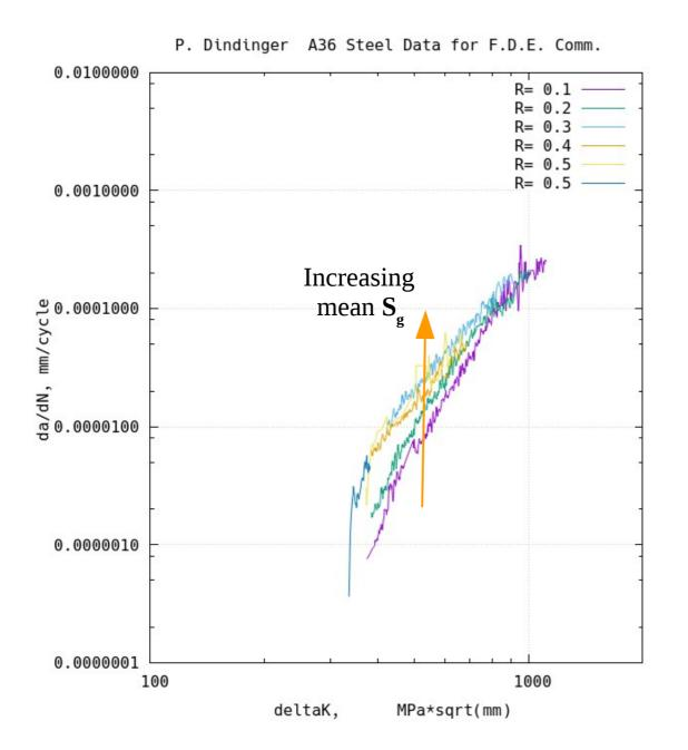
Mean stress effects are similar to those observed in crack initiation tests. With increasing tensile mean stress the da/dN curves move upwards and have a lower threshold  $K_{th}$
