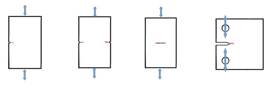
$K = F_1 * Sg \sqrt{\pi a}$   $K = F_2 * Sg \sqrt{\pi a}$   $K = F_3 * Sg \sqrt{\pi a}$
