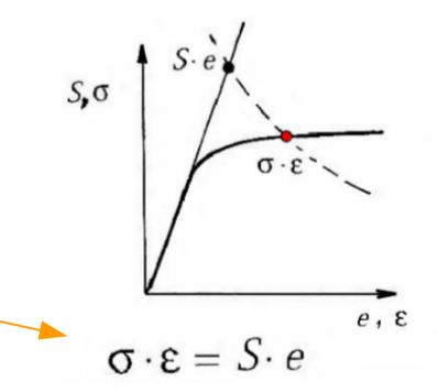
It can be solved by stepping along the "real" stress-strain curve in small increments, computing the energy at each step, and comparing the result to the elastic energy.
