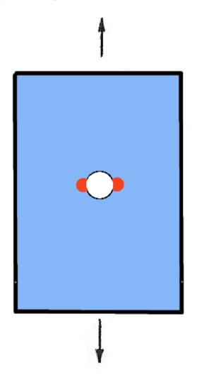
As the crack propagates, the plastic zone gets bigger, if +/-Sgross remains constant. At some point the net section will go fully plastic and the component will distort and become unusable.
