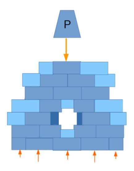
In the rough analog above the darker shaded bricks carry more load or stress.
