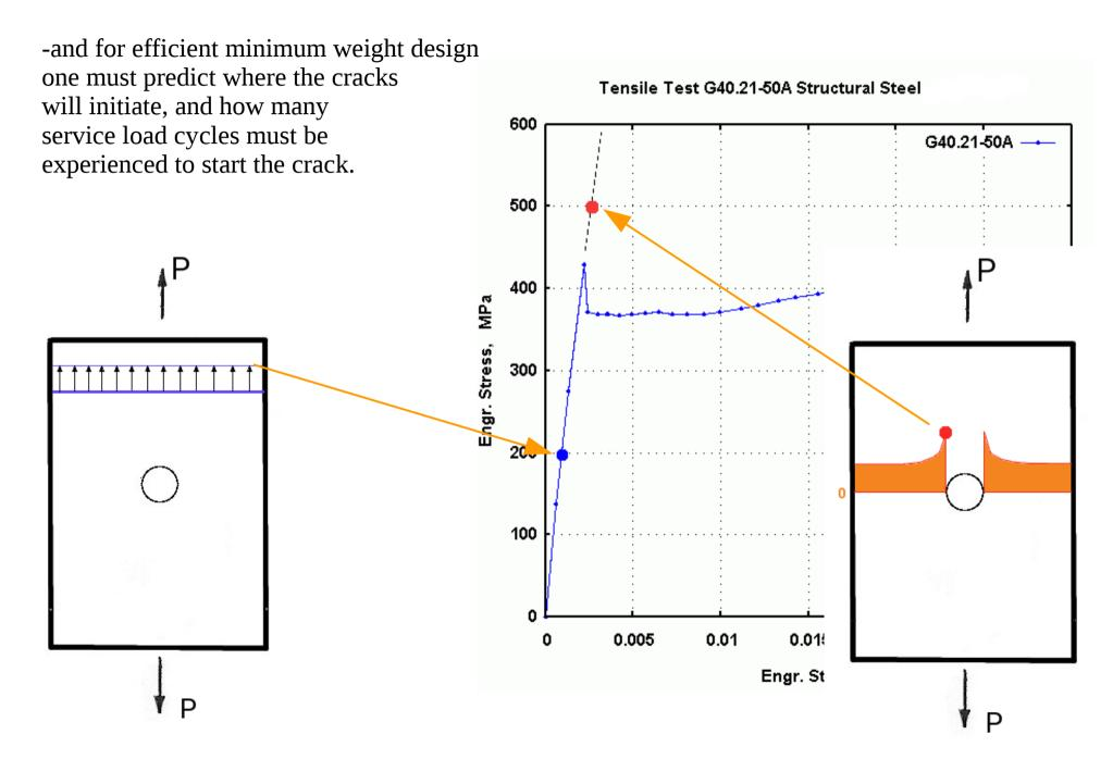
A small plastic zone (red) will not hurt a component that is mostly elastic(blue). The zone is constrained. The trade-off is that you may get a fatigue crack starting.
