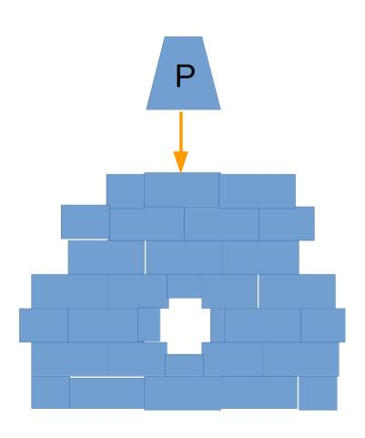
FEA represents a component or structure as a collection of "building blocks" They can have various shapes and sizes. In the rough example here we are using a bunch of elastic (rubbery) bricks that are glued to each other on all contacting sides.
