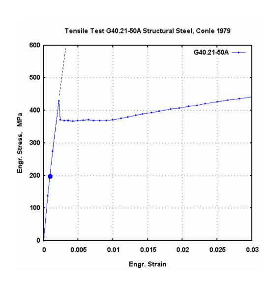
Fatigue cracks will start in such small plastic zones. Stress raisers are unavoidable.
