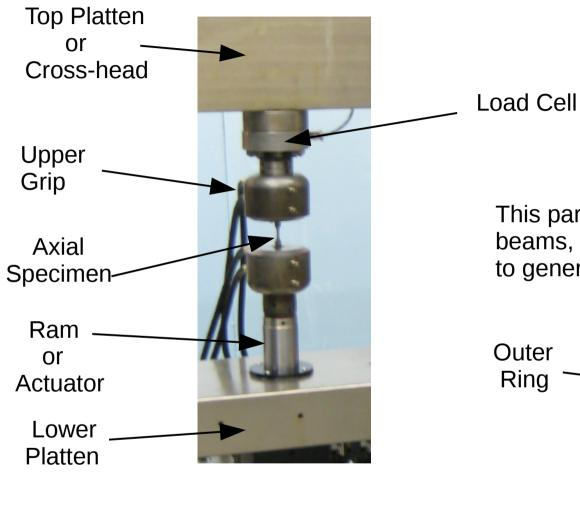
The deformation of membranes or beams are used to measure load in many load cells.
