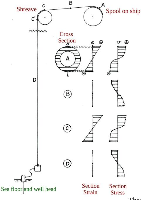
Coiled steel tubing is often used in the oil industry to service wells. In this off-shore example a large spool of coiled tubing is located on a ship and then un-rolled and lowered into the water down to the well head, where a connection is made and fluids are pumped in or withdrawn from the well.
