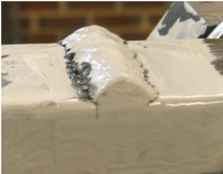
(3) Obvious Edge Crack
