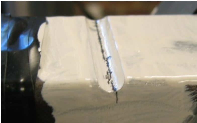
(3) Obvious Edge Crack
