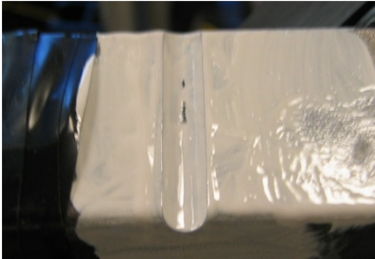
(1) First Crack Indication(s) Development
