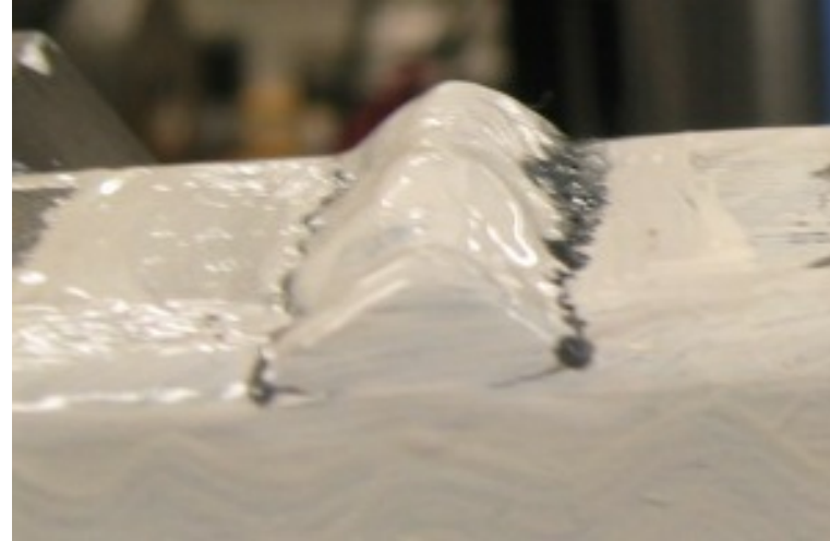
(2) Crack All the Way Across Width
