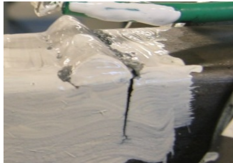
(4) Failure—Loss of Load Carrying Capability
