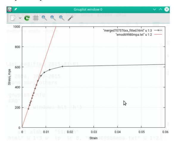
Step 4: For an elastic FEA stress of 650 mpa compute the equal energy (Stress \* Strain) on the cyclic curve.
