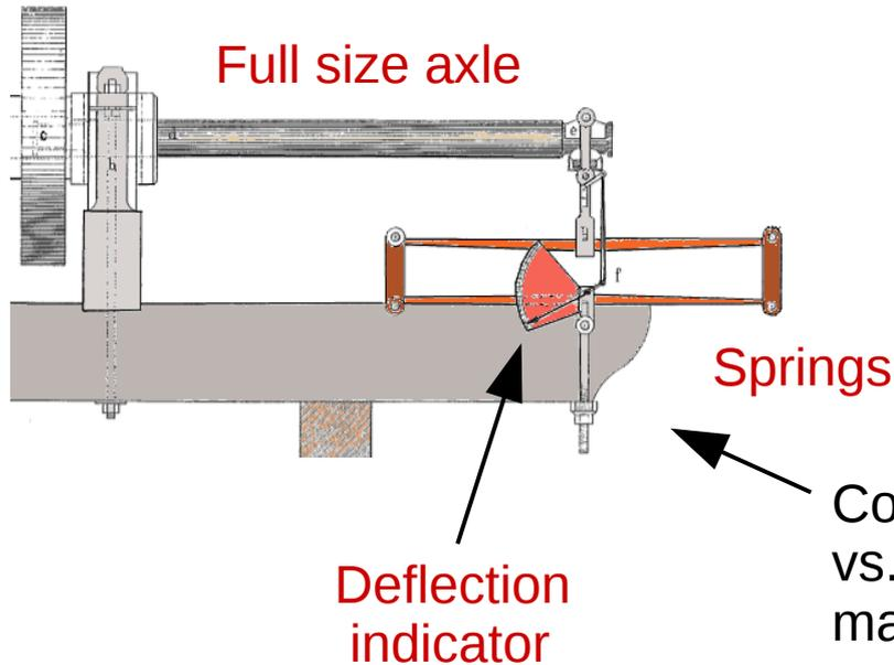
In Wöhler's axle test machine for example, the loads are applied by springs whose deflections have been calibrated with dead weights.
