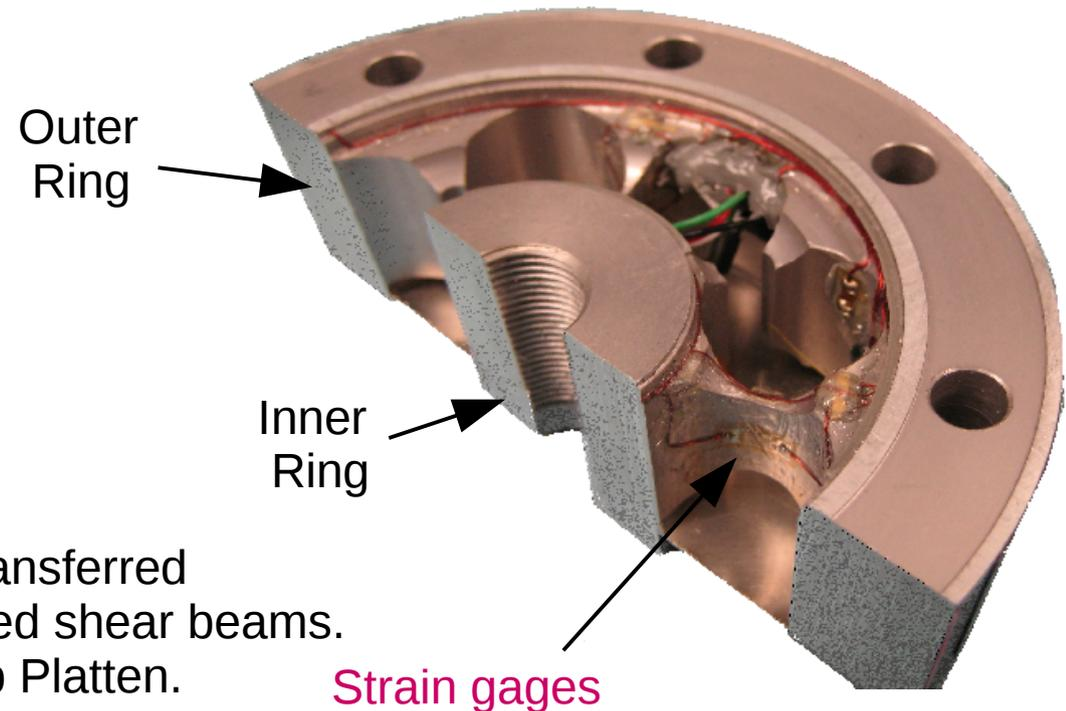
Load from the specimen entering the inner ring, is transferred to the outer ring by the gaged shear beams. Outer ring is attached to top Platten.
