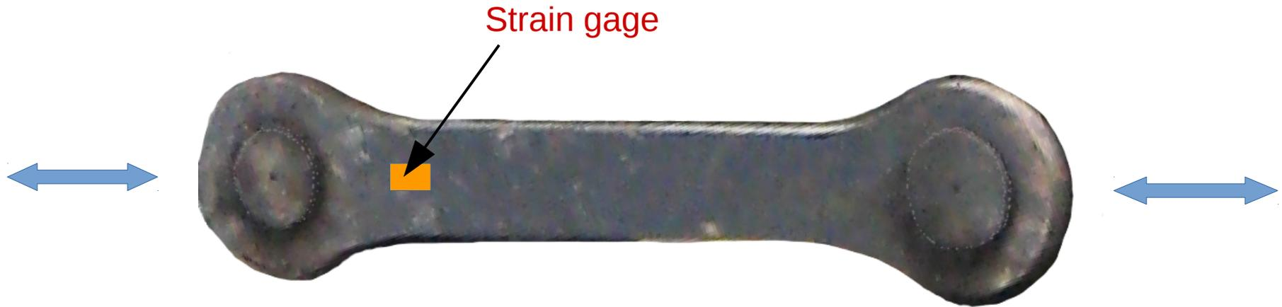
By attaching strain gages to components one can, with dead weight calibration, create a Load Cell.
